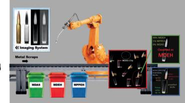
MetalScrap provides an automatic metallic scrap inspection approach utilizing advancements in X-ray technology, digital imaging, and advanced deep learning algorithms to provide an alternative metal scrap inspection method that can see through ammo-casing and is accurate, safe, and time-effective.
